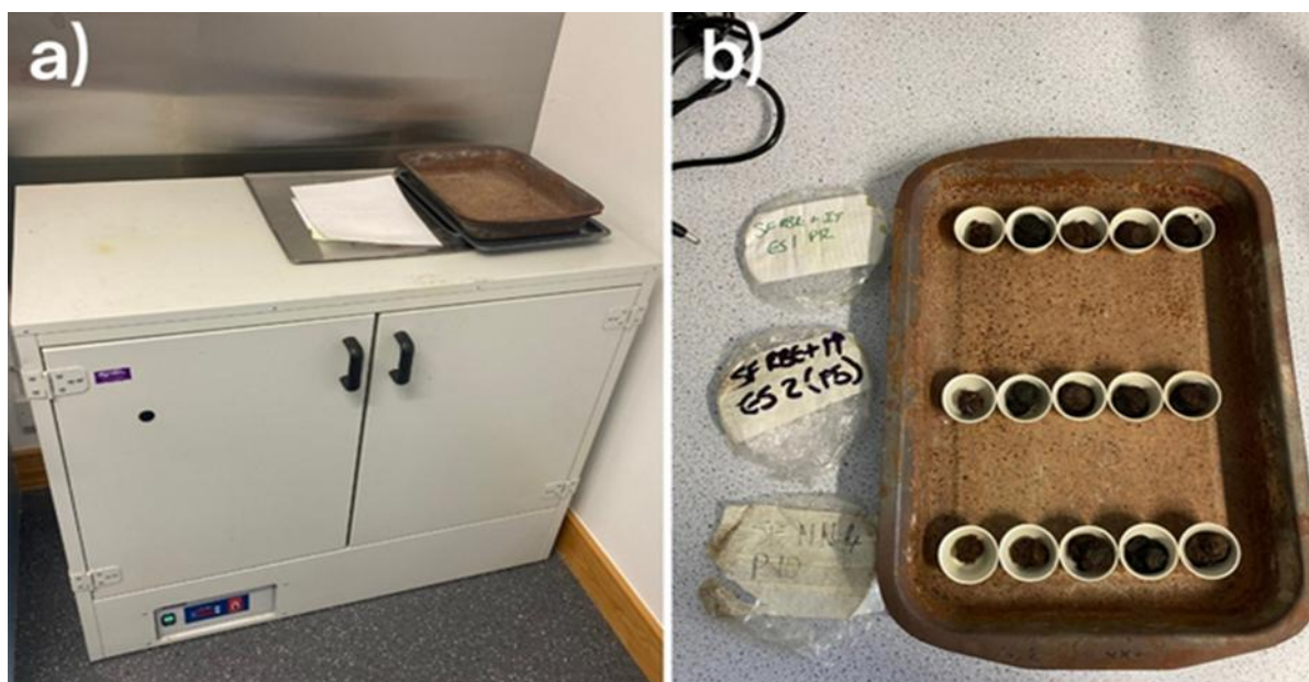
Figure 3.8: Laboratory assessments: a) Oven used to dry samples; b) wet sub-sample preparation example for oven-drying.
