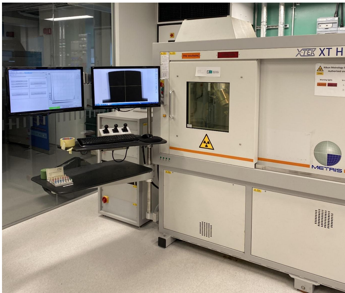
Figure 3.20: Nikon XTH 225 system used for alternative scans. Its smaller housing and reduced detector size limited FOV and geometric magnification.
