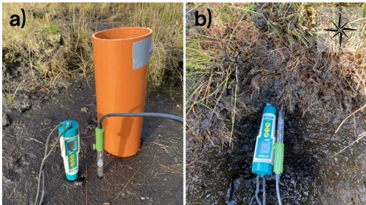
Figure 3.2: Field measurements: a) Surface (0cm) pH, Eh, and temperature assessments; b) Sub-surface pH, Eh, and temperature readings at 5cm intervals from the west-facing wall.
