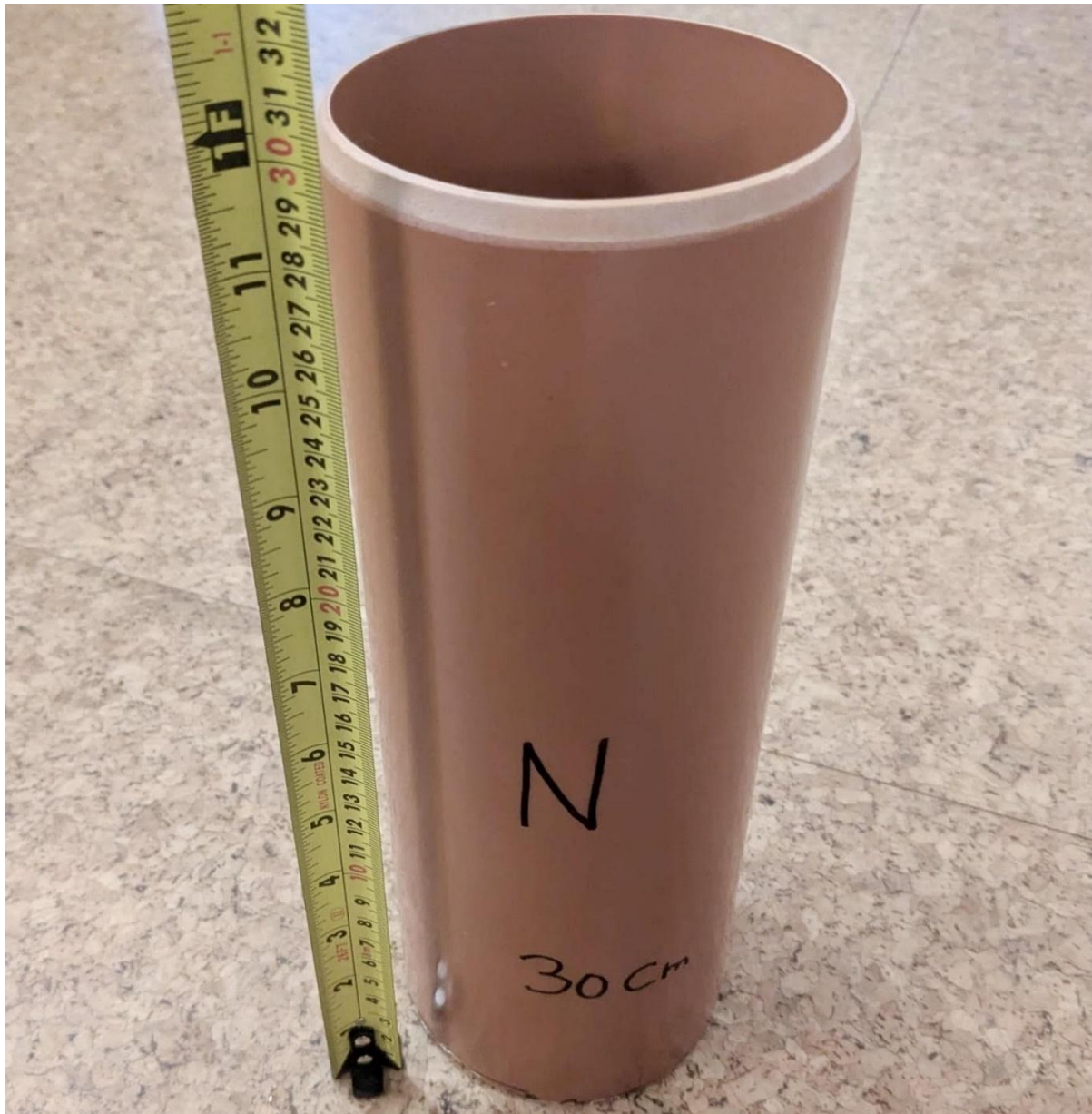
Figure 3.3: uPVC sample tube (110mm diameter x 300mm depth) used for undisturbed peat coring. The bottom edge (top of tube) is sharpened to aid insertion and minimise disturbance.
