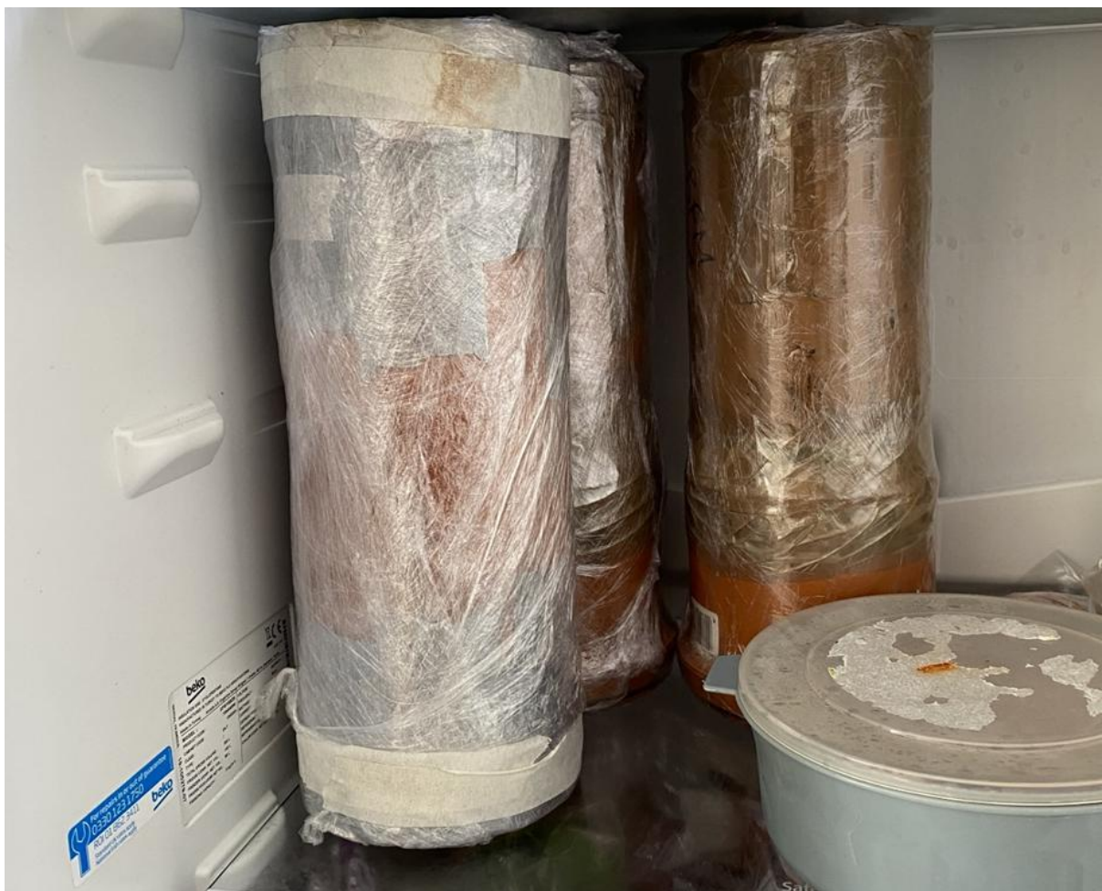
Figure 3.6: Vertical storage of extracted and sealed peat cores at 4°C prior to scanning and laboratory assessment.
