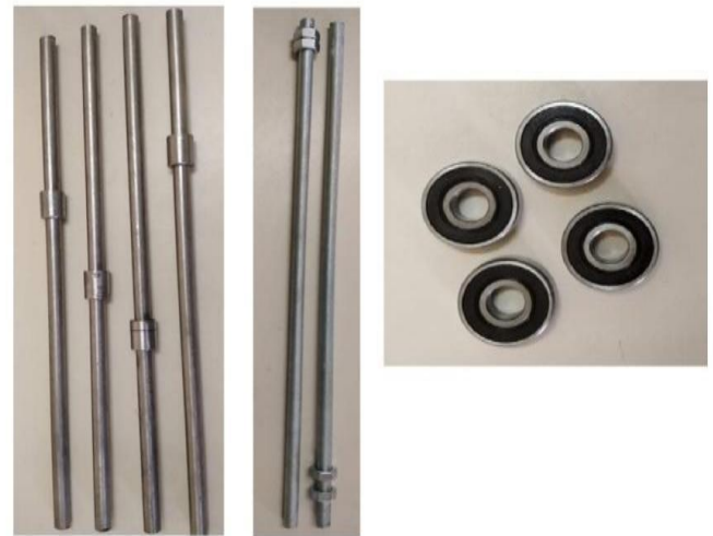
Fig. 1 shafts, screws, and ball bearings (12mm Diameter)
