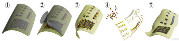
FIGURE 2. Dismantling sequence of a printed electronic to enable material recovery and reuse. Starting from a fully encapsulated device (1), the housing or laminate is removed (2) to access the functional printed layer (3). This layer is then separated into its key components: electronic parts/metal circuitry (4), and plastic substrate (5). These fractions can be processed and reintegrated into new materials.
