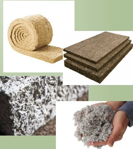
[Wool: top left; cork: top right; hempcrete: bottom left; cellulose: bottom right]
