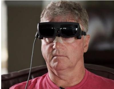
This is effectively an electronic “seeing aid” which amplifies the levels of light which fall on the eyes. It works particularly well in cases where visual acuity has been reduced through age, and is suited to use at night.
