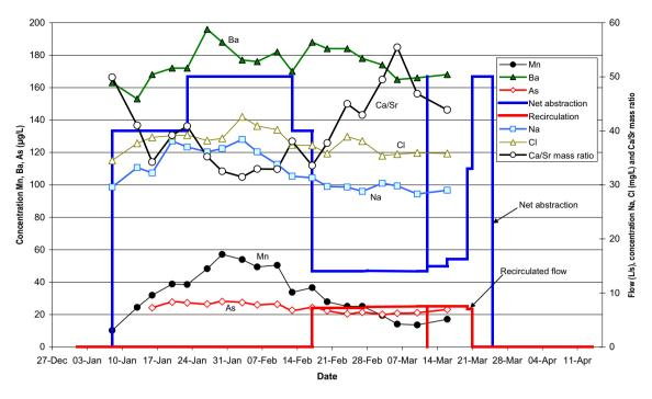
Fig. 7 Trends of key hydrochemical parameters (concentrations of chloride, sodium, dissolved manganese, arsenic, and barium) and the Ca/Sr mass ratio in the pumped mine water during the course of the Florence shaft pumping test
