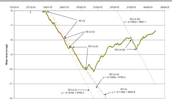
Fig. 10 Detail of water-level response to pumping in Florence shaft. *Trend lines* show best fit linear drawdown response to different episodes of constant rate net pumping at 40 or 50 L s<sup>-1</sup>
