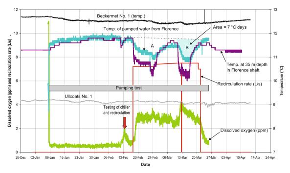
**Fig. 8** Temperature in shaft water column at 35 m bgl, temperature of pumped water, and dissolved oxygen content of pumped water, Florence shaft pumping test. *A* and *B* refer to the two periods of
