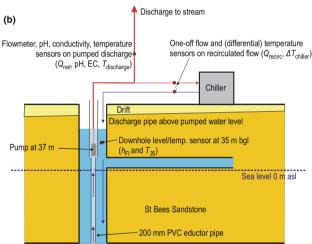
**Fig. 3** a Schematic cross section of Florence shaft, showing pumping test installation, **b** detail of upper portion of shaft. *m bgl* metres below ground level. *m asl* metres above sea level
