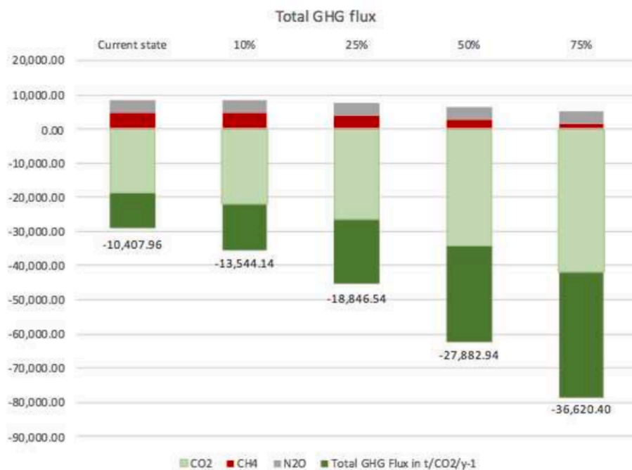
Fig. 4. Current state and alternative state total GHG flux final summary, incorporating CO 2 , CH 4 and N 2 O into the total flux assessment. The positive values indicate emissions and the negative values sequestration. Total sequestration in t/CO 2 /y -1 increases under each alternative scenario.
