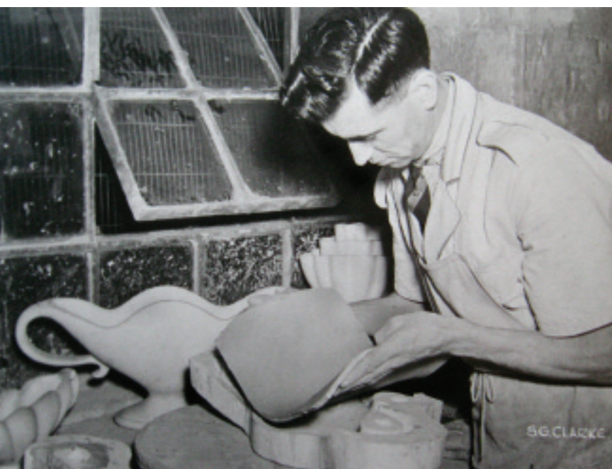
13. S.G. Clarke carefully lays a sheet of Devon clay into one half of an FMA mould prior to 'pressing'. Hammersmith & Fulham Archives and Local History Centre
