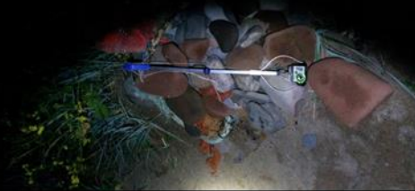
GoPro camera and custom made boom arm, River Gelt, August 2014
