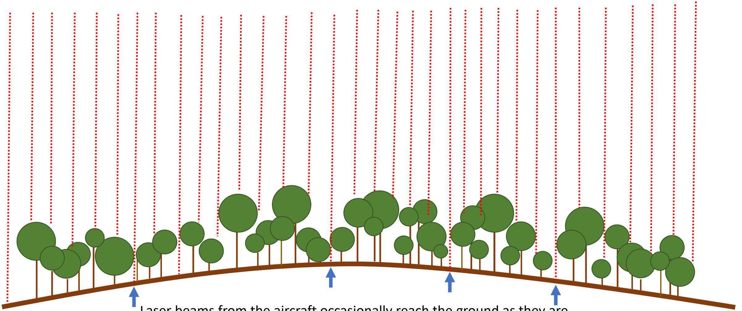
Laser beams from the aircraft occasionally reach the ground as they are only 12cm in diameter, and several thousand per second are transmitted.
