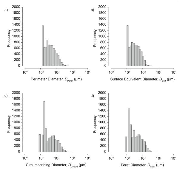
Fig. 4. Floc size distribution based on 3D data using equivalent floc diameter; (a) the  $D_{Feret}$ , (b) the  $D_{Surfb}$  (c) the  $D_{Circum}$  and (d) the  $D_{Perim}$
