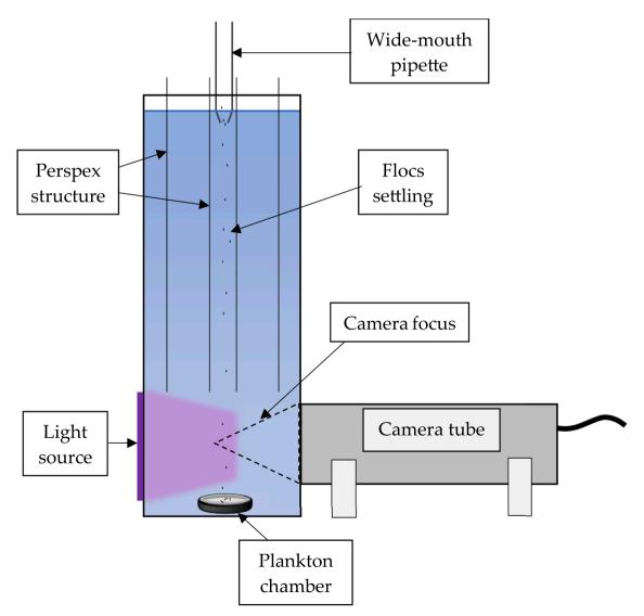
Fig. 1. Modified LabSFIOC settling column settling column and floc camera system.
