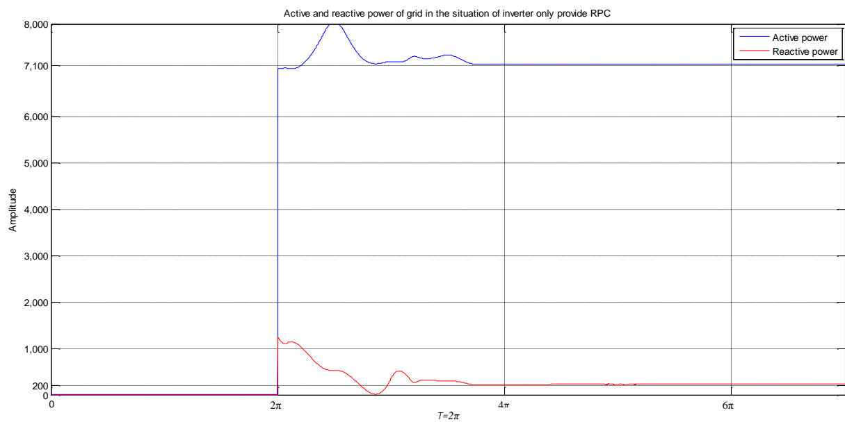
Figure 6- 20 Comparison of active and reactive power with RPC
