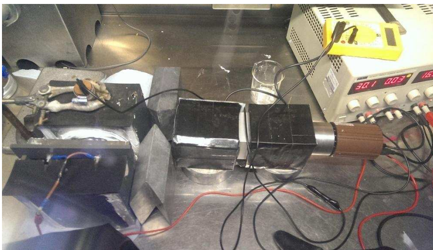
40 41 42 43 44 45 46 47 48 49 50 51 52 53 54 55 56 57 58 Figure 2. Photograph of the in situ CsI(Tl) detector setup used to monitor the decontamination of ^{137}\text{Cs} , where 59 the detector is surrounded with a lead collimator sheath with the circular aperture cut into the centre.
