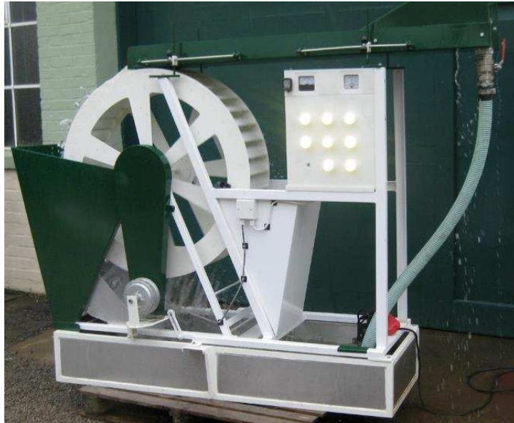
Figure 1: Prototype 1m diameter overshot waterwheel with water return by a submersible pump and connection to an LED lighting display.
