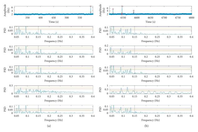
FIGURE 8: (a) Effect of a single short beat. (b) Effect of multiple errors.
