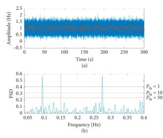
FIGURE 2: Signal masked by noise (solid line in upper graph) with 20% of RR intervals discarded at random (the remaining RR intervals appear as circles in upper graph). The frequencies of the original sinusoid are both accurately located at  $\omega_l = 0.095$  Hz and  $\omega_h = 0.275$  Hz and are the only peaks to exceed a FAP of 50% in the resulting periodogram. (a) Synthetic signal. (b) Lomb–Scargle spectrum.
