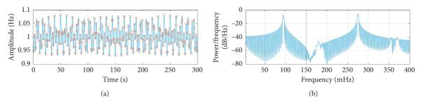
FIGURE 1: Synthetic data series with mean frequency of 1 Hz and zero phase, realized from the sum of two sinusoids via equation (4) with RR intervals (shown as circles) generated from (5) [12]. The resulting LS periodogram accurately locates peaks at  $\omega_l = 0.095$  Hz and  $\omega_h = 0.275$  Hz. (a) Synthetic signal. (b) Lomb–Scargle power spectral density estimate.
