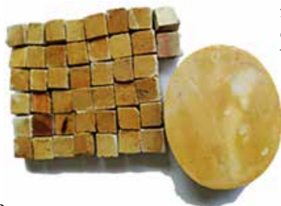
New tesserae cut from Giallo Siena Uniforme marble.
