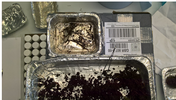
Figure 2.8: Forest of Ae. Roots were extracted from soil cores before soil was oven-dried at 105^{\circ}\text{C} .
