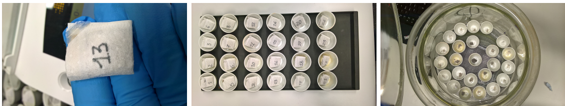
Figure 2.20: Clocaenog forest. Ash calculation after forage fibre analysis, from left: observation is folded and sealed before ashing; observations ready for ashing; observations ready for weighing after ashing: from batch n. 2 of the Ankom procedure. Outer circle crucibles contain observations from the L horizon of UN treatment. Inner circle crucibles contain observations from soil F horizon of CCF treatment. Note that ash is visibly more abundant in the F (CCF) horizon.
