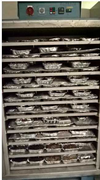
Figure 2.12: Forest of Ae. Soil samples were oven-dried at 35°C for 48 hours.
